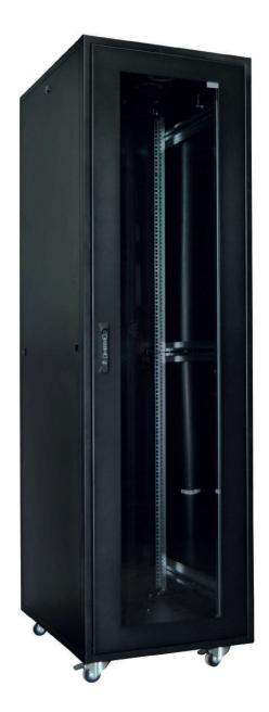
The standard Network Series Escab rack cabinet has got, leveling feet, the front door is single wing metal frame glass door by single point espagnolette locking system, removable solid metal rear cover with "O" ring locking system and spring hinged, sliding type cable entry at the bottom cover and vented top cover by knocked out blanking plate for cable entry as a standard product. Please check accessories for other alternatives.
